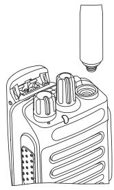
2 To remove the antenna, turn the antenna counterclockwise.
