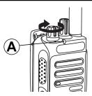
Rotate the **On/Off/Volume Control Knob** clockwise until you hear a click. You see MOTOTRBO (TM) on the display of the radio momentarily, followed by a welcome message.
