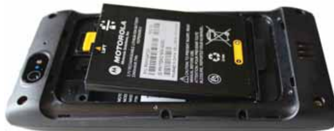
Figure 7: Installing the Battery
