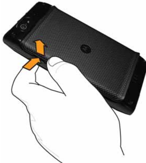
Figure 4: Removing the Battery Cover
