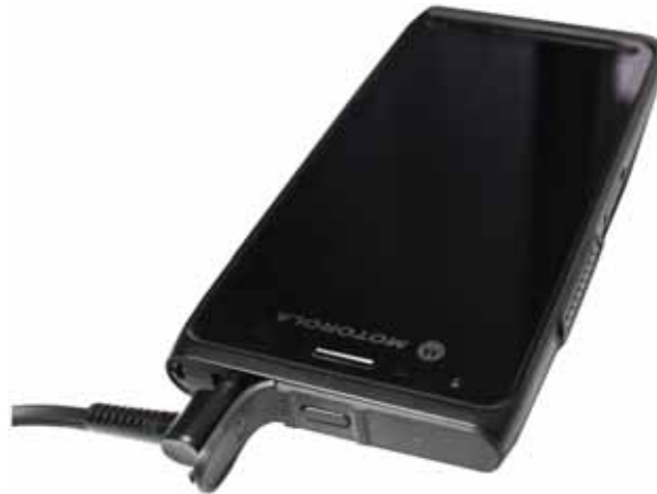
Figure 40: Insert Wired Headset Plug
