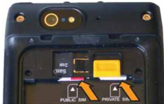
Figure 6: Installing the Public and Private SIM Cards
