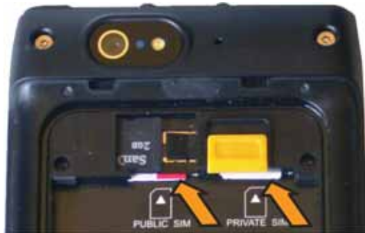
Figure 6: Installing the Public and Private SIM Cards
