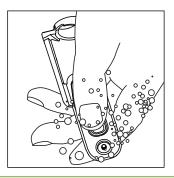
3 Use the toothbrush to scrub off any dirt or foreign matter from the niches of the top catch and thumb screw.
