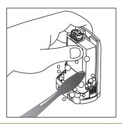
**5** Rinse the battery under running water to remove any excess detergent.
