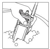
4 Lightly scrub the plastic area (front, back, bottom, top and side planes) of the radio with the small brush. Take extra care around the Speaker Grill and Microphone port openings.
