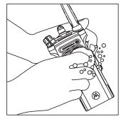
5 Use the toothbrush to lightly brush the gaps at the base of the knobs and around the switches. Take extra care around the Speaker Grill and Microphone port openings.
