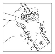
8 Shake off excess water and pat dry the radio with a dry towel. Take extra care to tap/shake out any trapped water from the speaker grill area.
