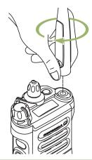
**3** To remove the antenna, turn the antenna counterclockwise.
