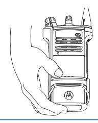
**4** Push at the bottom of the radio until the radio is released from it.
