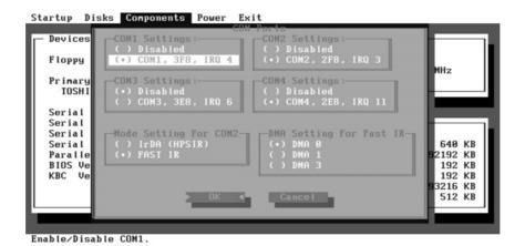
Allows you to configure the COM ports of the computer.
