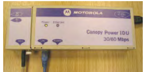
Figure 8: PIDU for 30/60-Mbps BH
