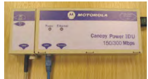
Figure 9: PIDU for 150/300-Mbps BH
