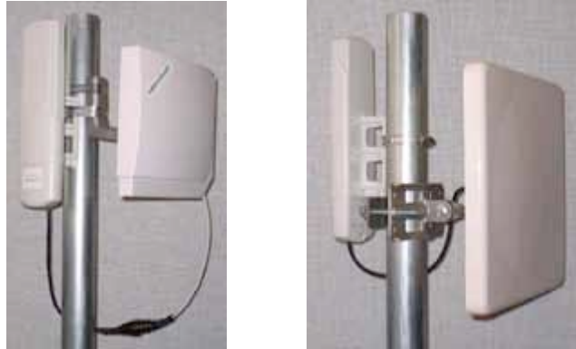
Figure 6: Examples of flat panel antennas with 900-MHz modules
