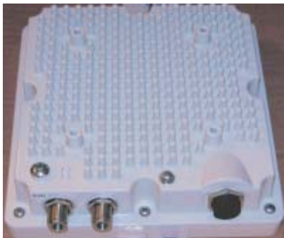
Figure 6-2 Connectorized CSM (CPE) 320 Rear View Connectors
