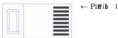
Figure 4-2 Pin 1 Location diagram
