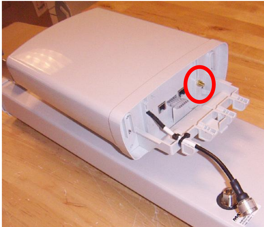
Figure 31: Ground lug highlighted on AP
