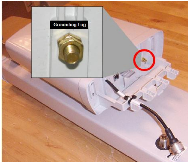
Figure 15: AP Grounding Lug
