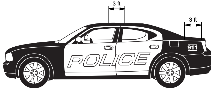
Figure 2-49. Multiple Antennas Separation
