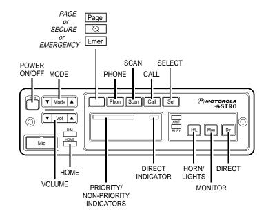
ASTRO<sup>®</sup> XTL<sup>™</sup> 5000 Digital Mobile Radio with W4, W5, W7, and W9 Control Heads User's Guide
