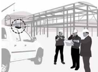
Figure 15a. Outdoors Temporary Repeater Installation Example
