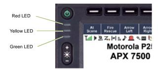
The LED lights up solid red while the radio is transmitting, and solid yellow when the radio is receiving a transmission (conventional mode only). There is no LED indication when the radio receives a transmission in trunking mode.
