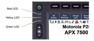
The LED lights up solid red while the radio is transmitting, and solid yellow when the radio is receiving a transmission (conventional mode only). There is no LED indication when the radio receives a transmission in trunking mode.
