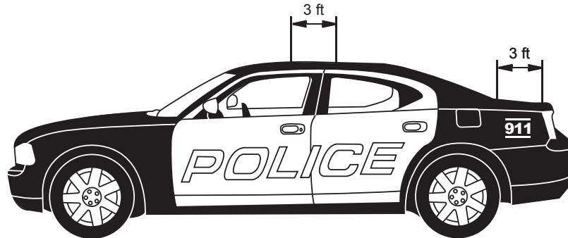
Figure 2-49. Multiple Antennas Separation
