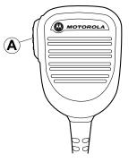
While a call is in progress, the PTT button allows the radio to transmit to other radios in the call.
