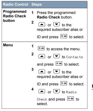
The display shows the Target Alias, indicating the request is in progress. The LED lights up solid green.
