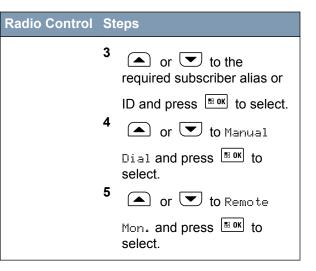
The first text line shows Rem. Monitor. The second text line displays the Target Alias, indicating the request is in progress. The LED lights up blinking green.
