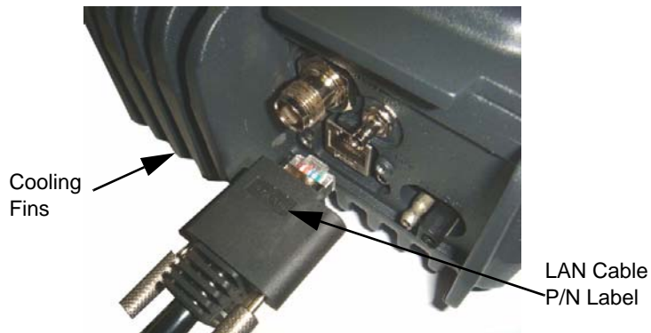
Figure 2-11 LAN Cable Connector Installation
