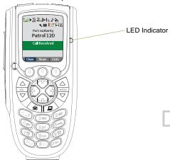
You see solid red while the radio is transmitting, and solid yellow when the radio is receiving a transmission (conventional mode only). There is no LED indication when the radio receives a transmission in trunking mode.
