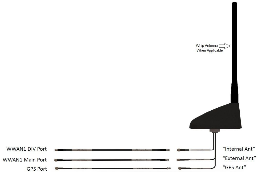
Figure 2-3 Antenna for Configuration Supporting LTE Private Network on WWAN1
