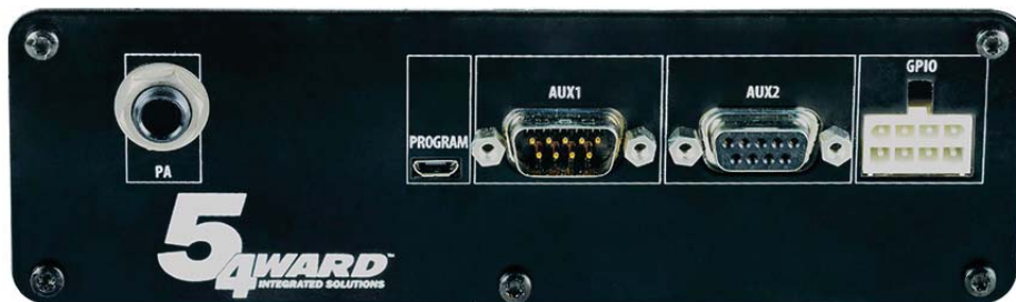
Figure 1-21. Siren and Lights Interface Module (SLIM)
