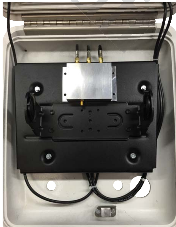
Figure 5-14. Multiplexer and Trunion Mounting
