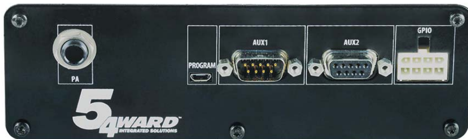
Figure 1-21. Siren and Lights Interface Module (SLIM)
