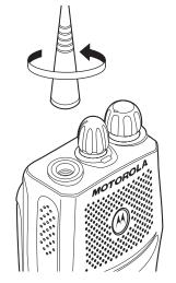
Turn the antenna counter-clockwise to remove it.
