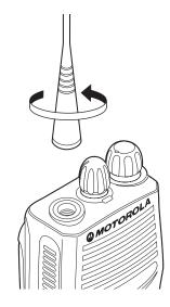
Turn the antenna clockwise to attach it.
