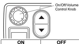
Rotate the **On/Off/ Volume Control** knob clockwise. If power-up is successful, you will hear the Self-Test Pass Tone ( \_\_\_\_\_\_) and see the green LED indicator and display icons light momentarily. If the radio fails to power up, you will hear the Self Test Fail Tone (\_\_\_\_\_\_). The radio will need to be returned
