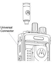
Insert the hooked end of the cover into the slots above the universal connector. Press downward on the cover to seat the lower tab properly into the RF connector.
