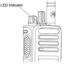
**Blinking red** – Radio is transmitting at low battery condition, receiving an emergency transmission or has failed the self-test upon powering up.
