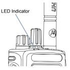
**NOTE:** The LED lights up solid green while the radio is transmitting and double blinks green when the radio is receiving a privacy-enabled call.
