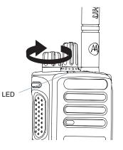
NOTE: The Home screen does not light up during a power up if the LED indicator is disabled (see *Turning the LED Indicator On or Off* on page 102).
