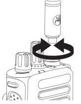
To remove the battery, turn the radio off. Move the battery latch into unlock position and hold, and slide the battery down and off the rails. To remove the antenna, turn the antenna counterclockwise.
