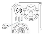
**NOTE:** The green LED lights up while the radio is transmitting and double blinks when the radio is receiving a privacy-enabled call.
