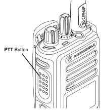
While a call is in progress, the PTT button allows the radio to transmit to other radios in the call.
