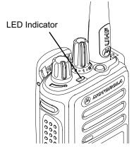
**Blinking red** – Radio is transmitting at low battery condition, receiving an emergency transmission, has failed the self-test upon powering up.
