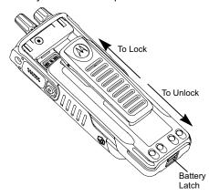
To remove the battery, turn the radio off. Move the battery latch into unlock position and hold, and slide the battery down and off the rails.
