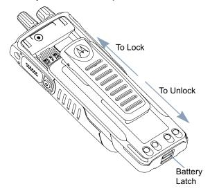
To remove the battery, turn the radio off. Move the battery latch into unlock position and hold, and slide the battery down and off the rails.
