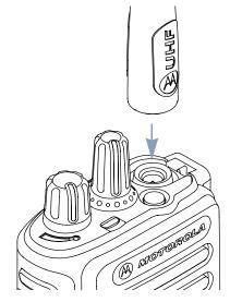
To remove the antenna, turn the antenna counterclockwise.
