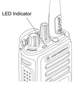
**Blinking red** – Radio is transmitting at low battery condition, receiving an emergency transmission, has failed the self-test upon powering up, or has moved out of range if radio is configured with Auto-Range Transponder System.
