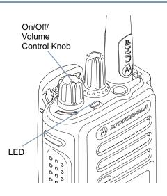
**NOTE:** The Home screen does not light up during a power up if the LED indicator is disabled (see Turning the LED Indicator On or Off on page 101).
