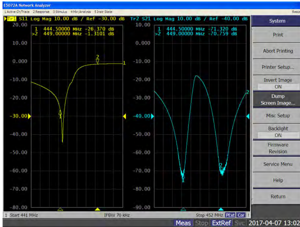
Figure 27: Rejection of Each Port for UHF Duplexer
