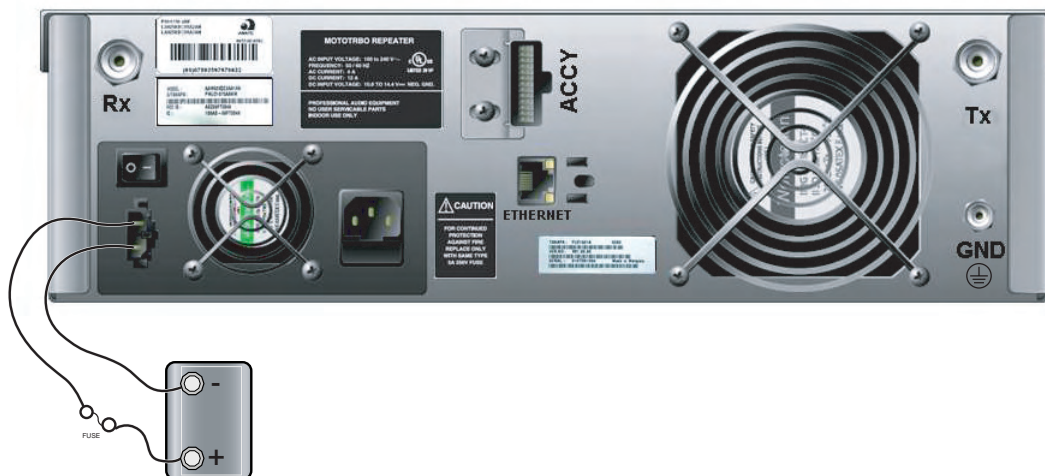
Figure 4-2 Making Connections to a Backup Battery
