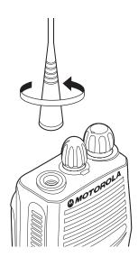
Turn the antenna clockwise to attach it.
