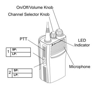
NOTE: Enter the functions for your radio's two programmable buttons in the boxes provided above. SP represents *Short Press*, while LP represents *Long Press*.
