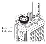
**NOTE:** The Home screen does not light up during a power-up if the LED indicator is disabled (see *Turning the LED Indicator On or Off* on page 46).
