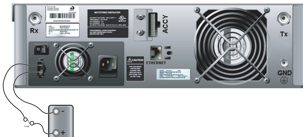
Figure 4-2 Making Connections to a Backup Battery
