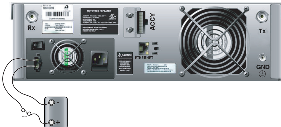
Figure 4-2 Making Connections to a Backup Battery
