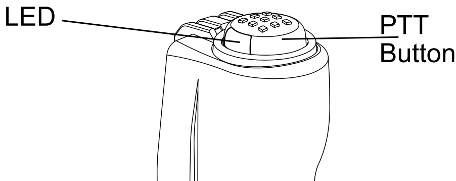
Figure 2 PTT Button and LED on the Bluetooth Adapter
