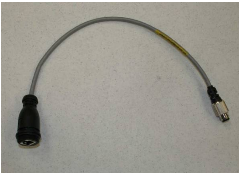
Figure 3-8 1ft Ethernet adapter cable (3063338B01)
