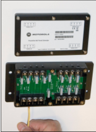
Figure 8 Wiring the Panel Extender
