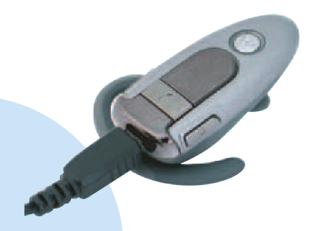
1 Plug the Motorola charger into the end of the headset.
