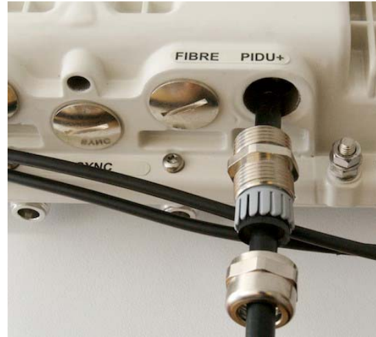
Step 2: Insert the RJ45 connector making sure that the locking tab snaps home
