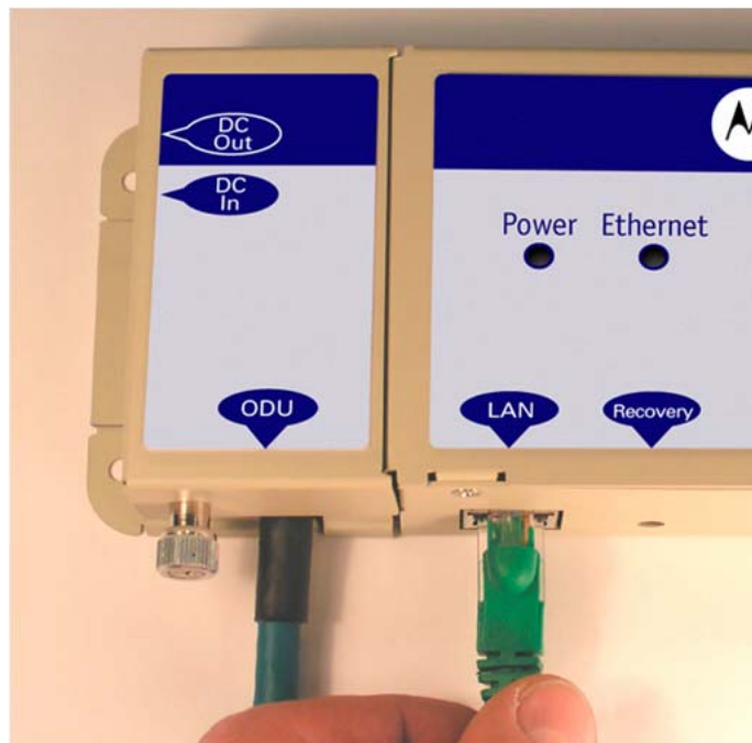
Figure 23 - Making the Network Connection at the PIDU Plus
