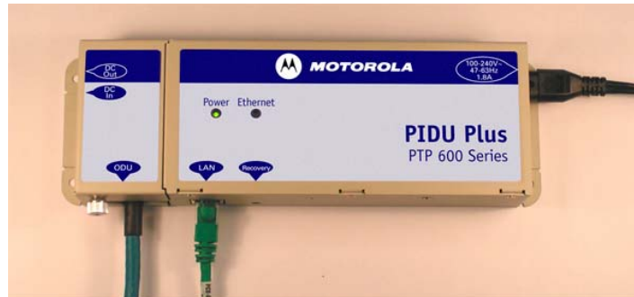
Figure 4 - Power Indoor Unit (PIDU Plus) – PTP 600 Series
