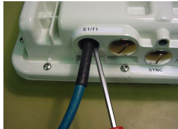
Figure 114 - Disconnecting the ODU
