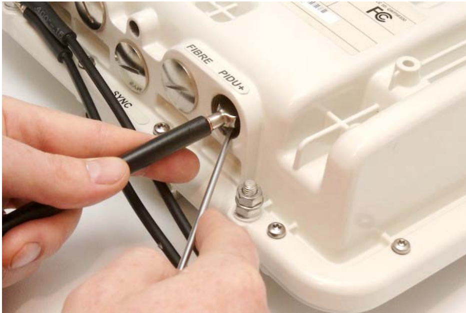
Figure 22 - Disconnecting the ODU
