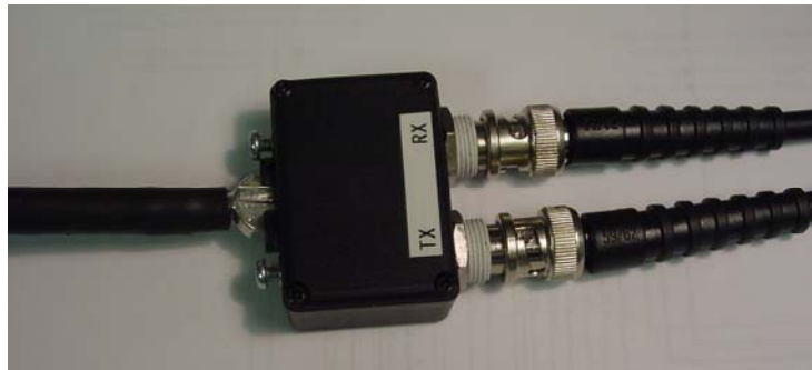
Figure 115 - Example of a Balun
