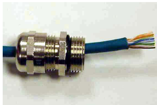
Step 3: Arrange conductors as shown in Figure 19 and cut to length
