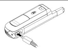
3. Insert the other end of the data cable into the data port of the other device.
