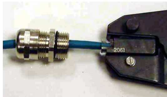
Step 4: Insert conductors and crimp
