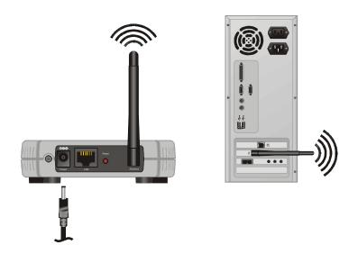
If you are connecting your client wirelessly to the access point, you can use the Motorola WPCI810G, a wireless PCI card for your desktop PC. If you have a laptop, the Motorola WN825G wireless PC card provides access.
