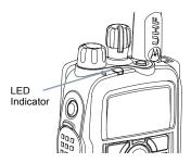
**NOTE**: The LED lights up solid green while the radio is transmitting and blinks green rapidly when the radio is receiving a privacy-enabled call.
