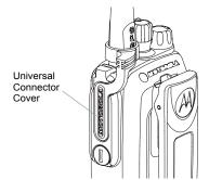
Place the universal connector cover loop over the attached antenna. Slide it all the way down to the base of the antenna.
