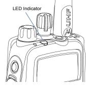
**Blinking yellow** – Radio is scanning for activity or receiving a Call Alert
