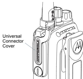
The universal connector is located on the antenna side of the radio. It is used to connect MOTOTRBO accessories to the radio.
