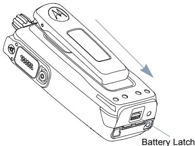
*To remove the battery, turn the radio off. Move the battery latch into unlock position and hold, and slide the battery down and off the rails.*
