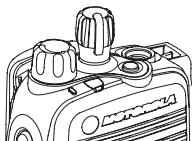
*To remove the antenna, turn the antenna counterclockwise. Make sure you turn off the radio and remove the universal connector cover first.*
