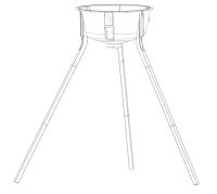
Align holes of hopper top, then press sides of hopper bottom until it snaps snugly in place. Insert bolt through each hole, place lock washer on bolt and screw wingnut onto bolt until tight. Repeat for all 12 bolts.
