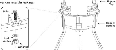
Connect Quick-Lock feeder kit to assembled hopper as shown.
