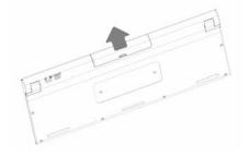
Install batteries with the positive (+) & negative (-) in the correct direction indicated by the AAA battery compartment label.
