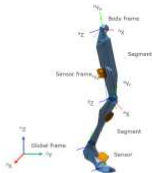
Figure 91: Global and local coordinate frames in MVN Analyze/Animate for the calculation of joint angles
