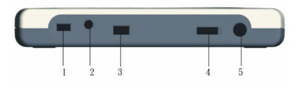
1 Power switch: switch to turn power on or off.
